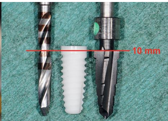
Fig 7: Pilot and profile drill: endosteal length 10mm plus 0.6 mm in the neck area.
